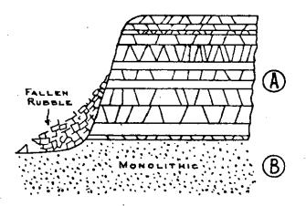
Underneath this group of strata there lies a softer rock B from which stone can be cut up to any manageable size, say up to 10 ft.  $\times 10$  ft.  $\times 5$  ft.
