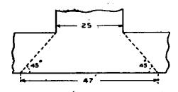
Loads.—Weight of block (submerged) at 88 lb.  $100 \times 47 \times 11' \times 88$  lb. =2,035 tons.
