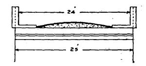
on a width of 24 ft.=1×60×24×100=144,000 lb. 18,720 Add to live load 13 p.c. per Farr's Rule to bring as 162,720 lb. to equivalent dead load' .. •• . .
