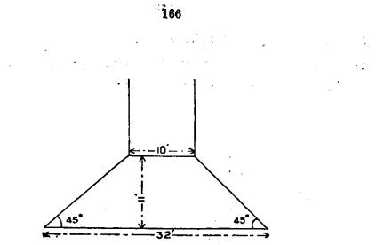
Supposing weight spreads at an angle of 45°.
