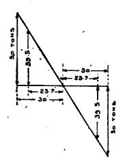
The value of shearing stress varies uniformly from 50 tons at end to zero at centre of 39.5
