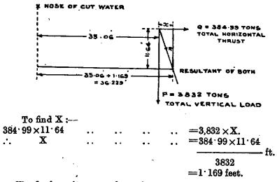
... The final resultant cuts base of pier at distance 35.06+1.169 ft. =36.229 feet from nose of cut water.
